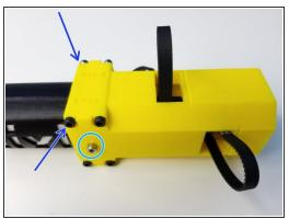
Place the GT-2 Timing Belts around the Small Pulley Gears
