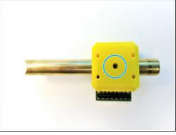
Mount the AS5147 Sensor on the <u>Sensor Holder</u> using the M2 Screws
